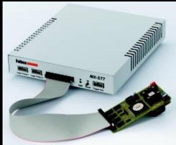
Consists of a “pod” that holds or replaces the processor and a “chassis” that contains specialized debugging hardware, including a trace buffer.
