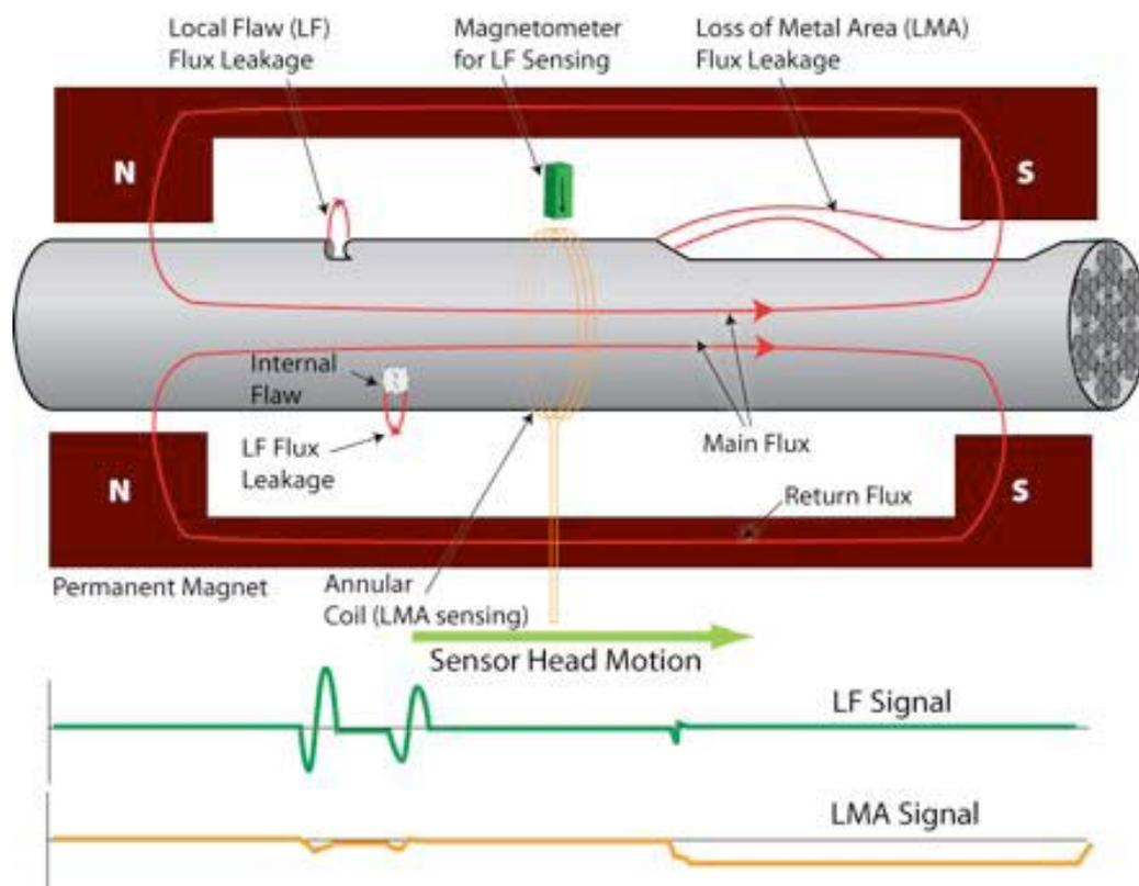
**FIGURE 3 - Sectional cut through magnetizing sensor head and idealized measurements representing idealized defects in wire rope [Courtesy of Tethers Unlimited, Inc.]**
