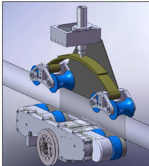
**FIGURE 6 - Cutaway schematic view of guy crawler**
