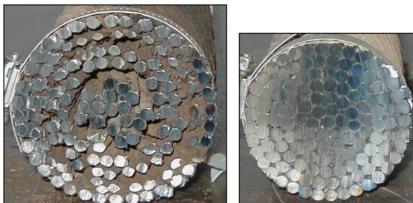
**FIGURE 2 - Comparison of internally corroded versus uncorroded sections of same guy**
