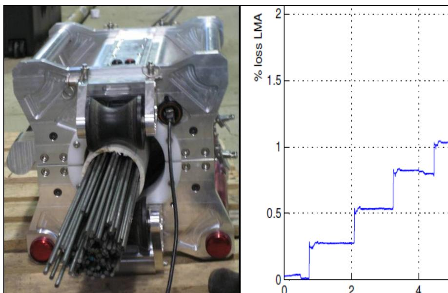
**FIGURE 5 - Magnetizing sensor head undergoing standard rod reference test**
