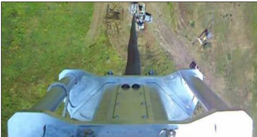
**FIGURE 7 - View from the rear of the robotic crawler about half way up the guy**
