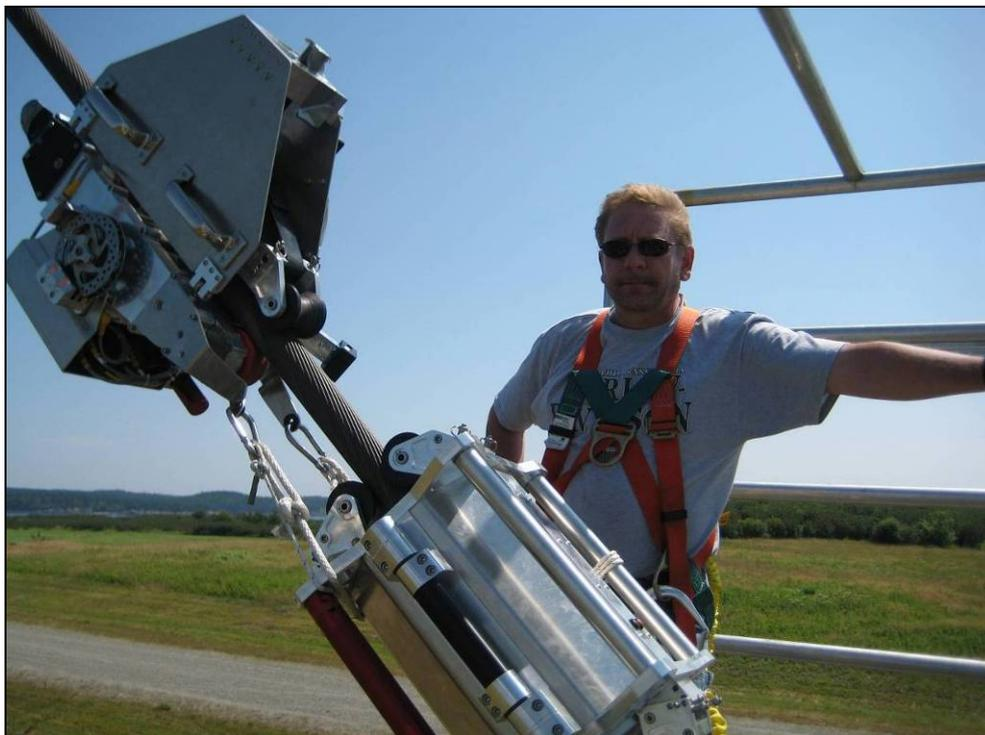
**FIGURE 4 - Guy Crawler towing magnetizing sensor head on tower guy**
