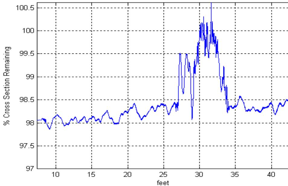
**FIGURE 9 - Measured gain in cross-sectional metallic area across artificial defects**
