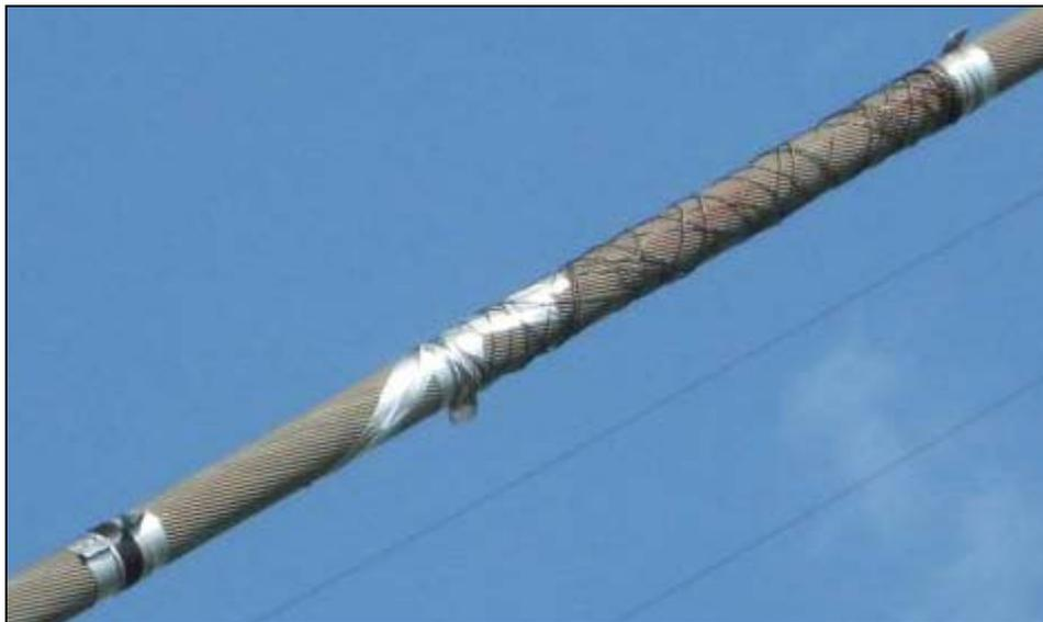
**FIGURE 8 - Artificial defects added to the guy for testing tool sensitivity**
